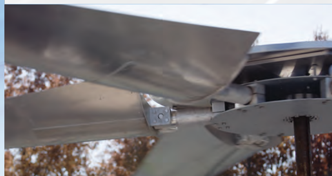
5052 marine grade aluminum blade
